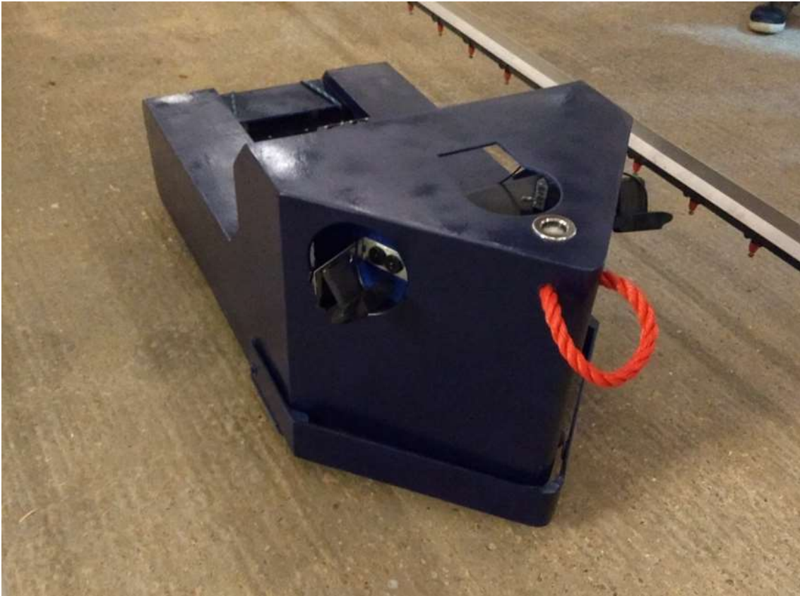
Figure 2: Photograph of the robot and cover used for the trial.. Dimensions: L 1060 mm x H 465 mm x W 520 mm
