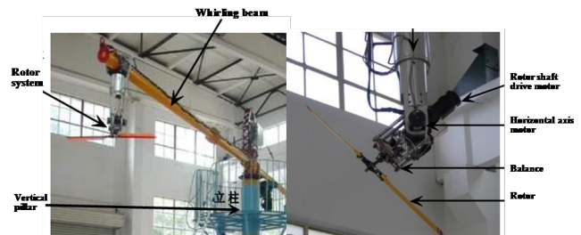
Figure 6. The whirling-beam rotor maneuvering flight test rig
