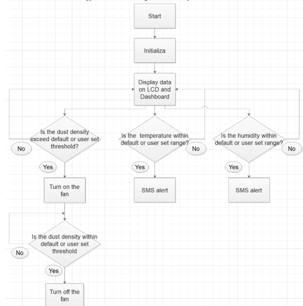
Figure 2. System Control Logic
