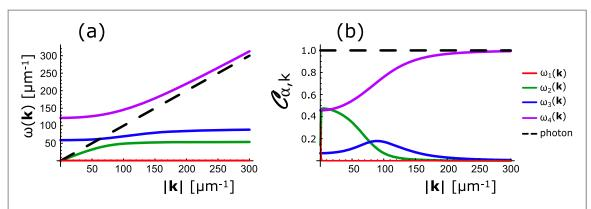
**Figure 1.** (a) Polariton branches of fused silica (solid) in units of c=1, as well as free photon dispersion (dashed). Note that the optical regime lies between 3–20  $\mu$ m<sup>-1</sup>, whereas the majority of the structure in the spectrum is at higher energy. (b) Overlap coefficient  $C_{\mathbf{k}\alpha}$  for the different branches. Note that the value varies between zero and unity depending on whether a specific branch  $\alpha$  can be characterised as 'photon-like' or not.
