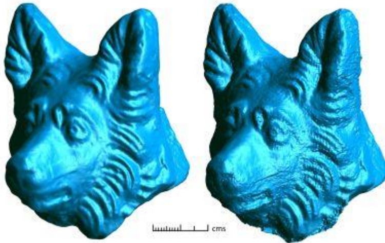
Figure 2: Comparison between Romer laser scan data (left) and Metashape photogrammetry data (right). The model derived from photogrammetry data shows good dimensional accuracy and yet has very poor detail reproduction. The ribbed effect to the surface on the right hand side, for instance, is not present on the original. © Lloyd Bosworth
