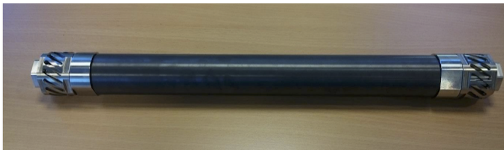
(a) The Ceratec main reactor body reactor.
