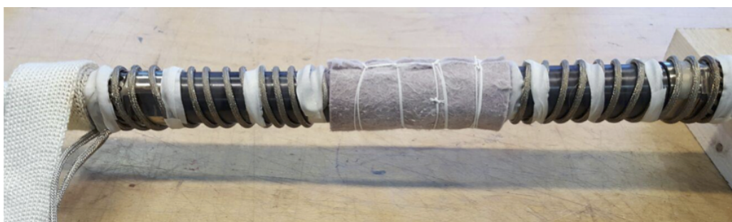
(b) Reactor traced with the first layer of thermal insulation.
