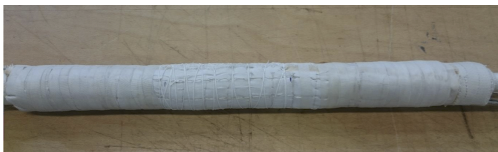
(c) The fully insulated reactor, ready to be inserted in the magnet.
