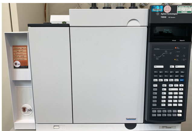
Figure 6.14 The Agilent GC: 7890-0378 - Three Channel Fast Refinery Gas Analyser.
