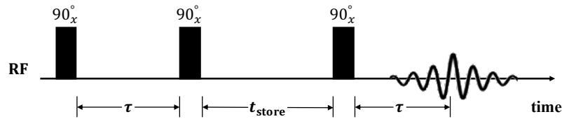
Figure 3.12 The stimulated echo pulse sequence where refocusing of the spin phases is achieved by two extra consecutive 90^\circ pulses.
