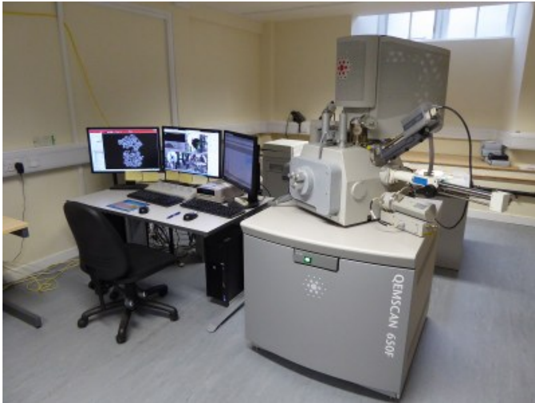
Figure 4-21 Thermo Scientific Quanta-650F at University of Cambridge Earth Science department was instrumental for imaging of my uranium dioxide thin film samples.
