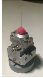
Figure 4-12 Capillary sample shown mounted on goniometer used to align the capillary with the beam. The lower circular part allows the goniometer to be screwed to the diffractometer.
