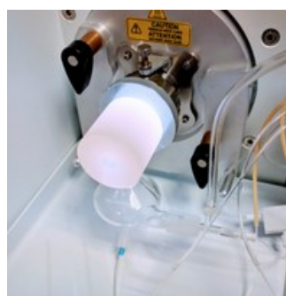
Figure 4-19 The left figure shows the schematic of the flow of ions and the right figure shows the argon plasma generated to ionise the aqueous sample.
