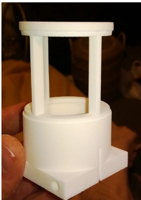
Figure 4-11 Guard made to mount on the goniometer and protect the capillary which was to align with the windows. In use these were sealed with Kapton film.
