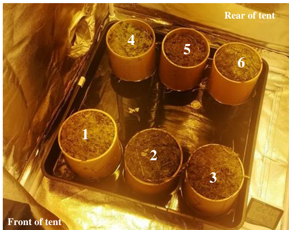
Figure 3.2: Sphagnum and peat cores in gas collars placed in tray on 17/01/2019. Sample numbering system shown.
