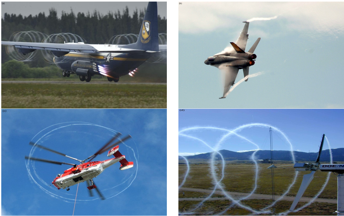
Figure 1.1: Helical vortices created from different devices such as from a: (a) propeller [63]; (b) wing [176]; (c) rotor [27]; and (d) blade [38].
