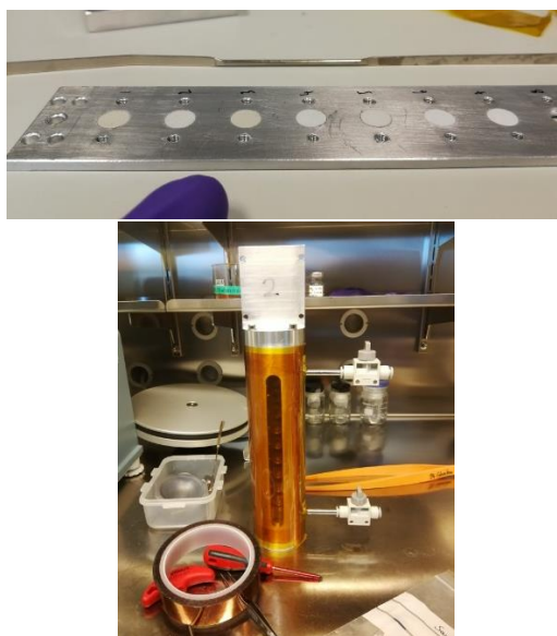
Figure 9: Air tight cell used for XAS analysis at B18, Diamond Light Source
