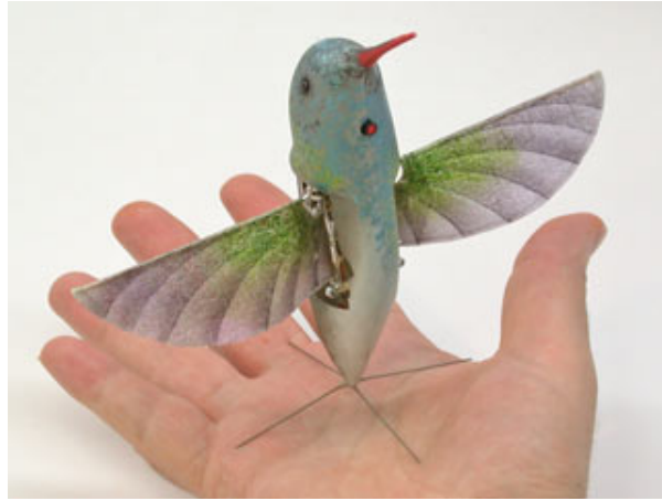
Fig. 1.3. Nanohummingbird, a flapping wing Miniature-aerial-vehicle developed by Aerovironment Inc.
