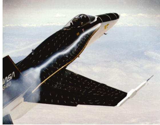
(b) Vortices on the F18-HARV in flight [4].
