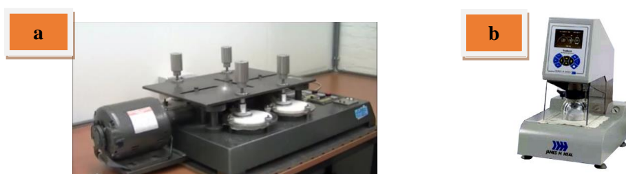
Figure 5.1 Image of James H. Heal Martindale (a) and James H. Heal & Sons Truburst burst tester (b) used for abrasion and burst strength testing, respectively (James Heal, 2014)
