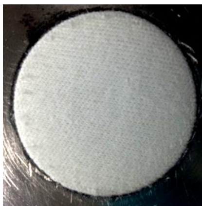
Figure 5.3 Abraded cotton sample treated with MTES only sol and padded once at pad pressure 15 kg/cm after 30,000 revolutions
