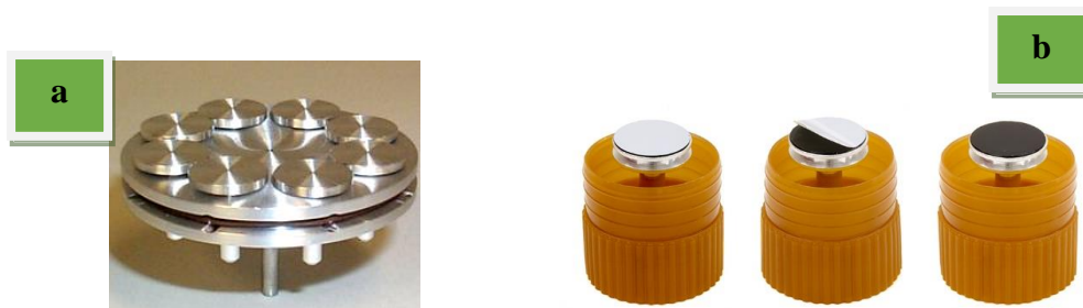
Figure 6.4 Examples of carousel sample holders without adhesive tape (a) (E. Fjeld Company, 2003) and SEM aluminium stubs and adhesive tape (b) (Emresolutions, 2014) used to hold samples for SEM analysis
