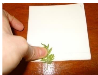
Figure 39. Pressing on leaf to deposit trichome content onto TLC plate.
