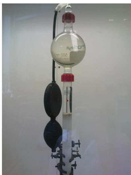
Figure 43. Flash column, used to separate deoxyartemisinin from artemisinin
