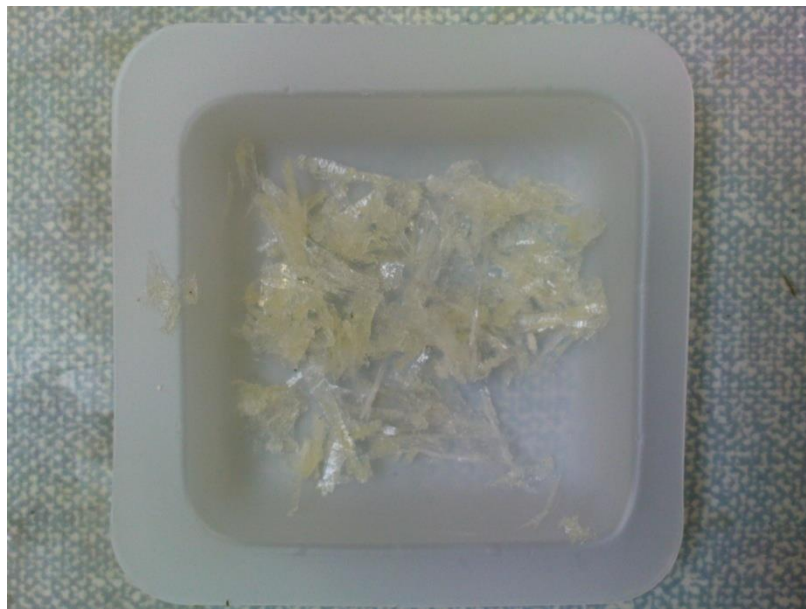
Figure 44. Impure crystals containing both deoxyartemisinin and artemisinin.
