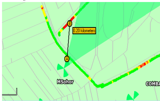
Gambar 4.13 Bad Spot Ec/No Site PTK114MW1_MSOHORMW1
