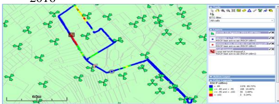
Gambar 4.2 Coverage Plot RSCP 8 Agustus 2016 Sumber : Data Hasil Pengukuran Nemo Analyze
