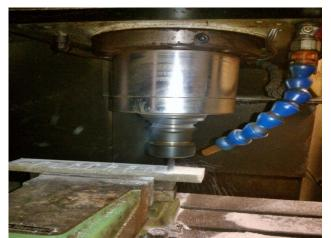
Figure 1: Machining of GFRP by CNC vertical machining center with K10 carbide End Mill
