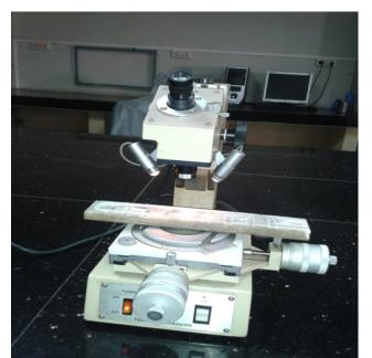
Figure 3: Measurement of delamination damage using Tool makers Microscope
