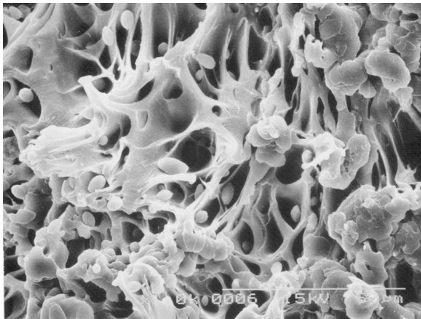
Figure 3: SEM image of PET/5.0%LCP blends without PMDA reactive additive. Room temperature fracture is accompanied by plastic flow around poor adhering LCP fillers
