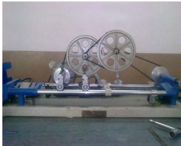
Figure 6: Digital Tensometer attached with capacitive type displacement transducer (Mikrotech, Bangalore, model: METM2000ER1)
