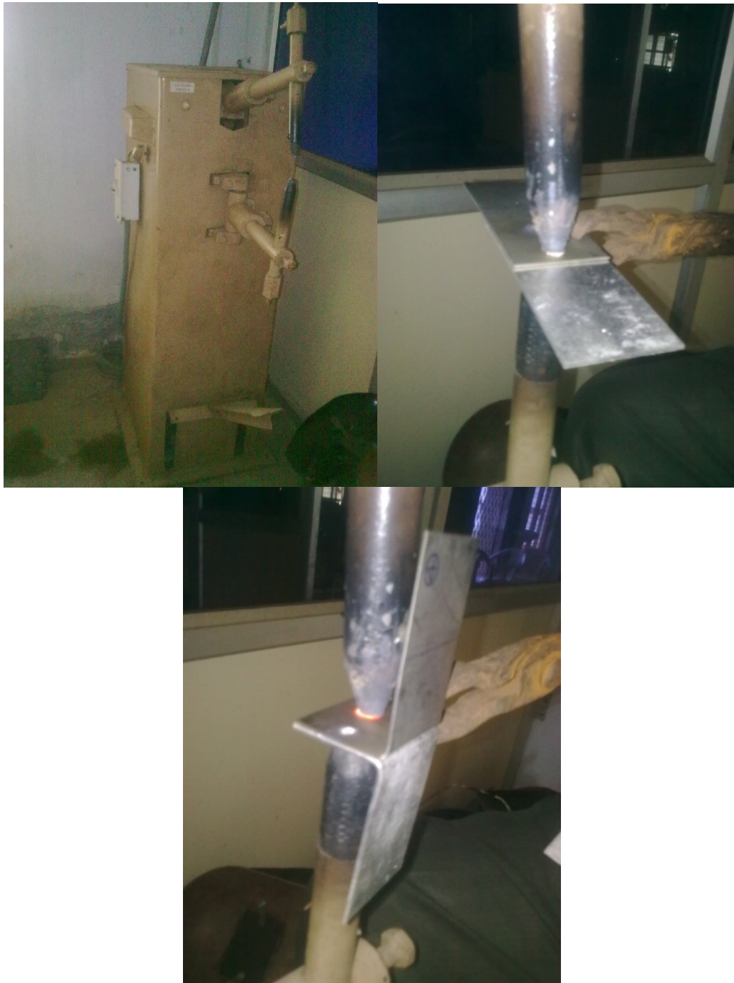
Figure 5: Resistance Spot Welding Equipment (pedestal type) & Specimens during resistance spot welding for lap and T-joints
