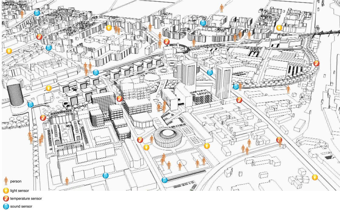
Figure 1: A sketch of a city where fixed sensors are found as part of the infrastructure and people walk around possibly carrying sensing devices. The combination of both fixed and mobile devices forms a SNoS.
