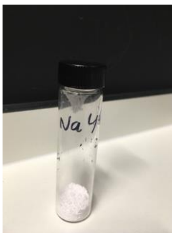
Figure 36: \text{NaYF}_4: \text{Er}^{3+}, \text{Yb}^{3+} powder in a vessel. Unlike the \text{Sr}_4\text{Al}_{14}\text{O}_{25}: \text{Eu}^{2+}, \text{Dy}^{3+} sample, it did not exhibit phosphorescence once the lights had been turned off after exposure to sunlight, so the lifetimes of its photoexcited states are much shorter.
