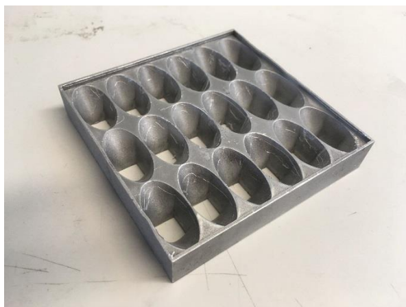
Figure 89: Image of the metal casting mould used to produce a batch of SEH concentrators.
