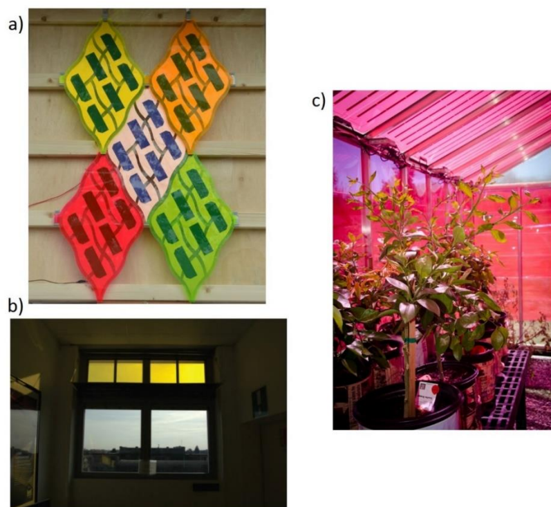
Figure 30: Examples of real LSC-PV modules for applications in BIPV: (a) Roof Leaf module design [237], (b) smart window powered by yellow LSC-PV [236] and (c) greenhouse made from red LSC-PV [238].
