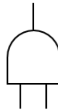
AND gate: the output occurs only if all the inputs occur (inputs are independent).
