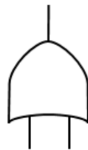
OR gate: the output occurs if any input occurs.
