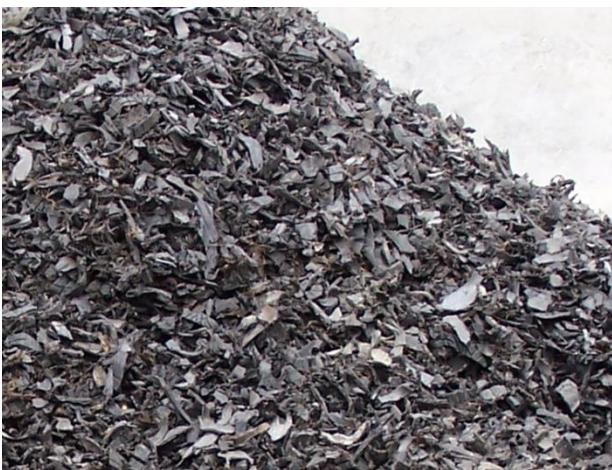
Fig. 3. Shredded exhausted tires (image at 1m scale).
