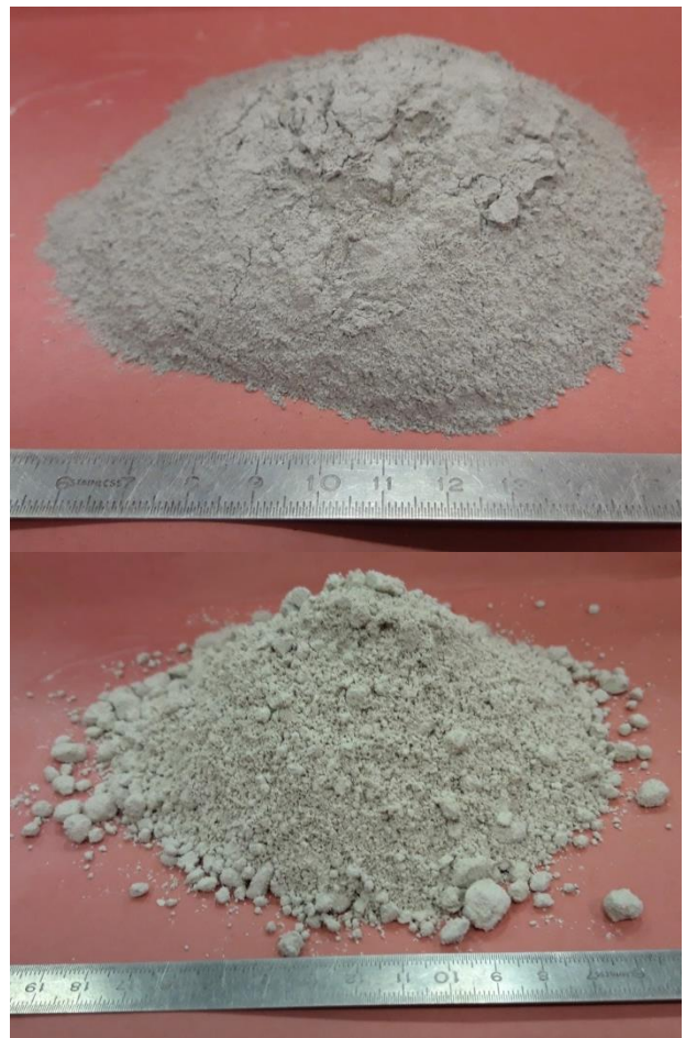
Fig. 5. Fine powder from quarrying/mining activities currently not recycled. (Top) from dry comminution process of olivine minerals. (Bottom) from wet comminution of quartz minerals (credits Oggeri 2019).
