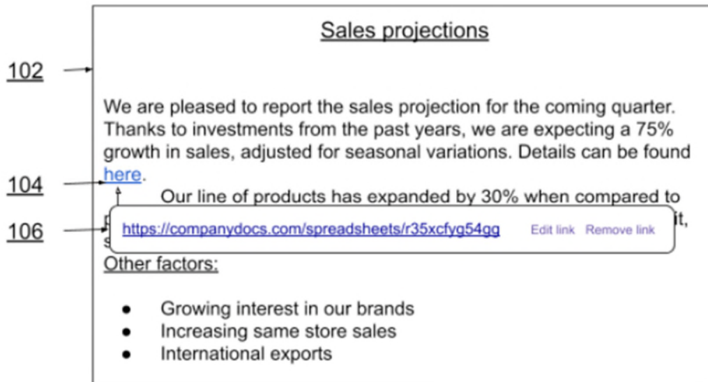
Fig. 1: A floating window provides an expanded version of a link within a document
