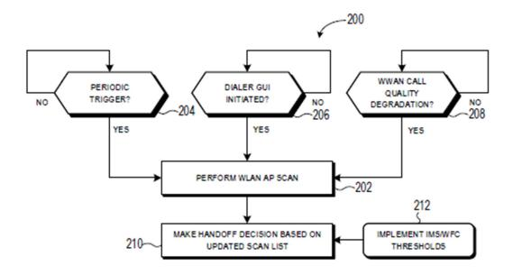
FIG. 2 – adaptive WLAN AP monitoring process
