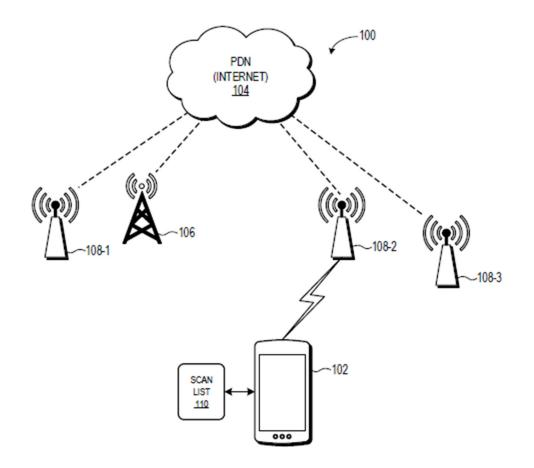
FIG. 1 – mobile cellular system employing adaptive WLAN AP scanning
