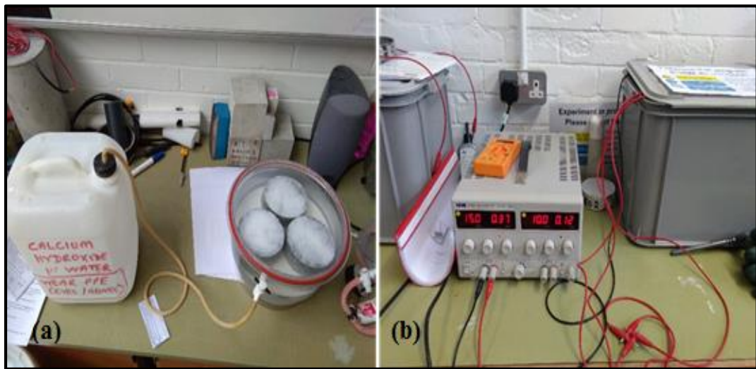
Figure 6.7. (a) Immersed specimens in saturated \text{Ca}(\text{OH})_2 , (b) RCPT montage
