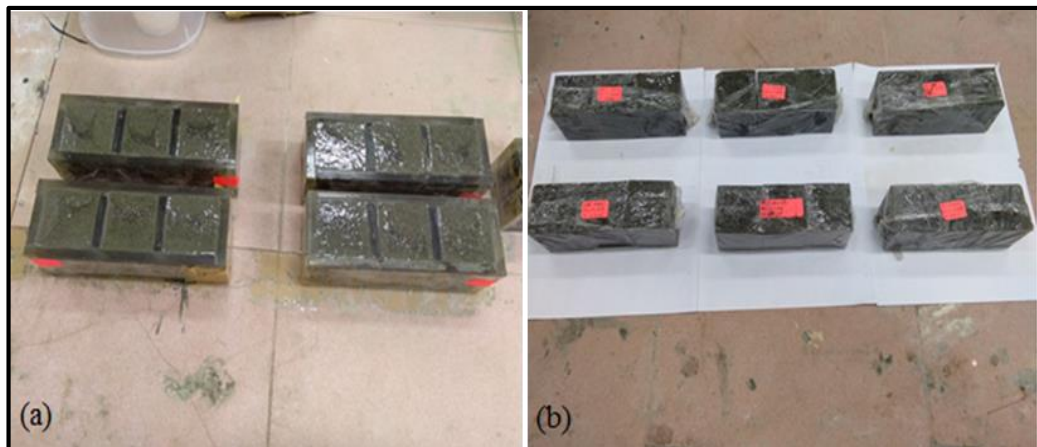
Figure 3.6. GP Paste specimens a); Fresh b); Hardened
