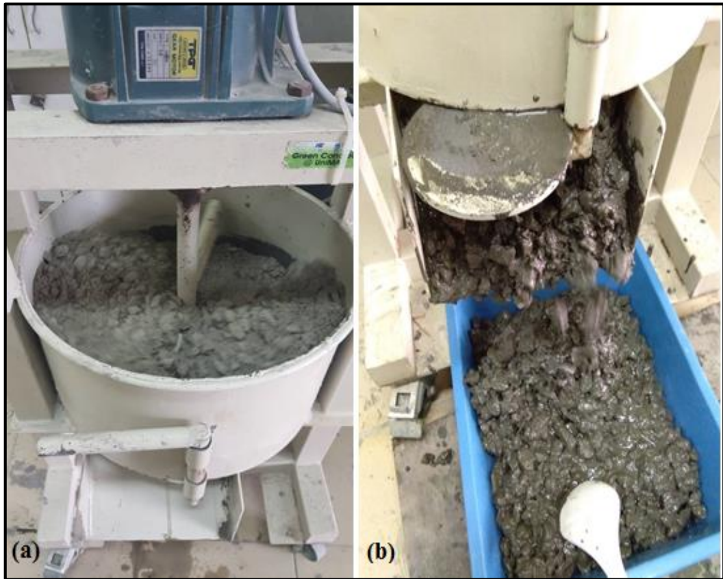
Figure 3.7. (a) Dry mix, (b) Fresh GPC mix
