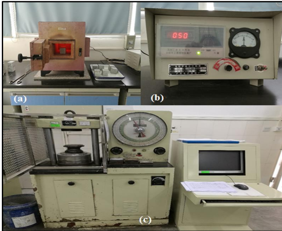
Figure 7.2. (a) Electrical Oven, (b) Auto-temperature regulator, (c) Universal mechanical machine
