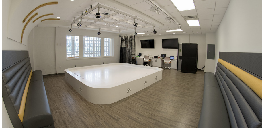
Figure 7.1: The Robotarium, a remotely accessible swarm robotics tested, allows users to remotely upload code which gets executed on a team of physical differential-drive robots [151]. In addition to these robots, the hardware infrastructure of the Robotarium consists of an elevated arena where the robots operate, a motion capture system seen attached to the roof above the arena, and wireless chargers embedded into the walls of the arena.
