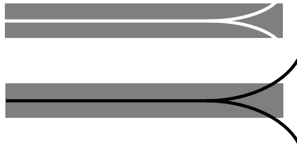
Figure 11-5. Schematic of guided insertion method, pre (top) and post (bottom) anchor rod insertion.
