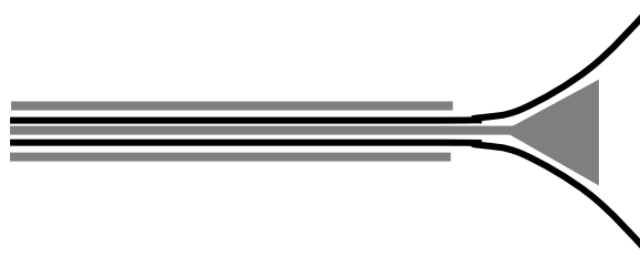
Figure 11-4. Schematic of wedge method for installation of root-inspired anchor.
