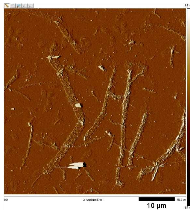
Figure 2.15. AFM amplitude images of bubbles after drop-cast drying on the glass slide.
