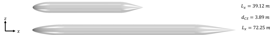
Fig. 18 Experiment 5: comparisons 1-4 assess the impacts of detailed fuselage shape parameters, while comparisons 5-8 establish the significance of cross sectional area and overall fuselage length
