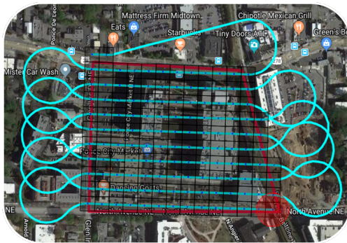
Fig. 4 Dubins path - used for manned aircraft
