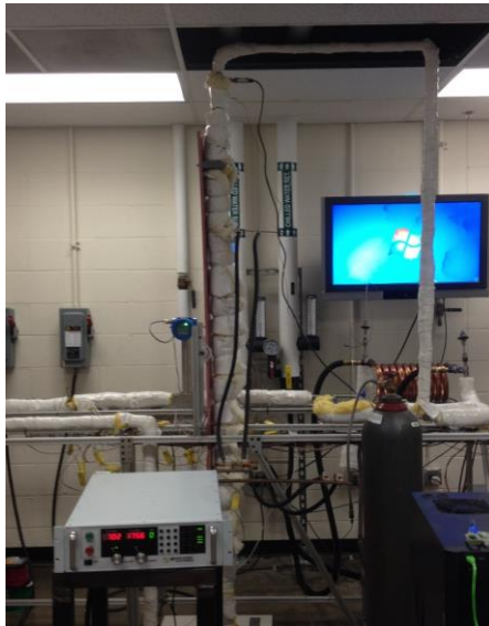
Figure 3-4: Picture of the test facility showing the circular tube test section installed in vertical upward orientation
