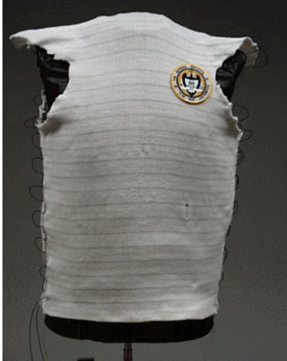
Figure 6-10 Front View of First Generation Knitted Sensate Liner
