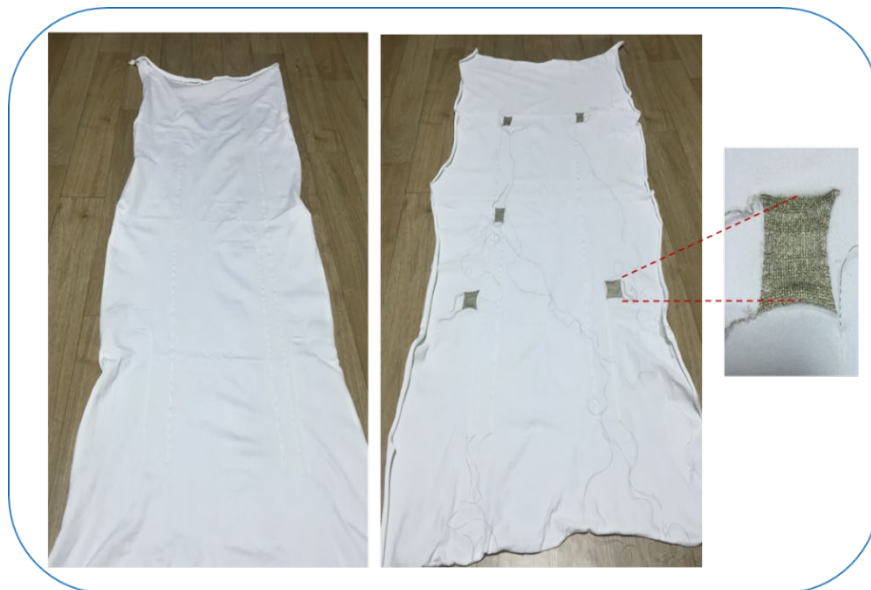
Figure 8-6. Fabric with Integrated Sensors and Data buses
