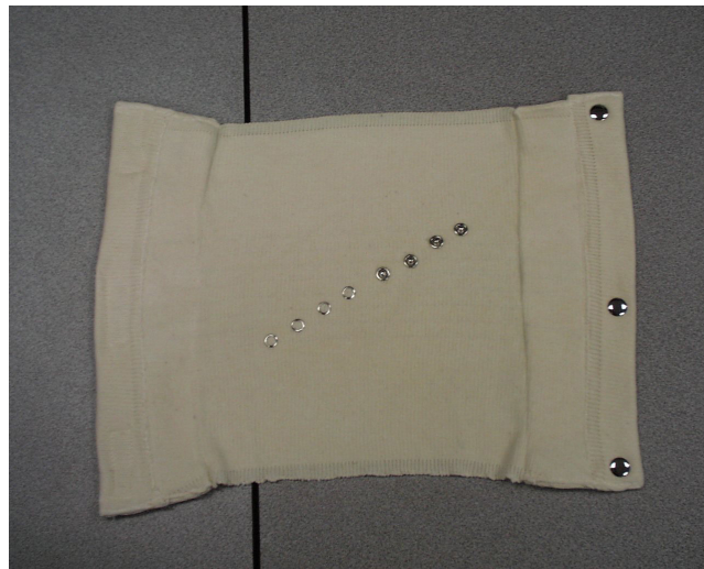
Figure 6-13 Sensate Liner Sample for Launderability Test
