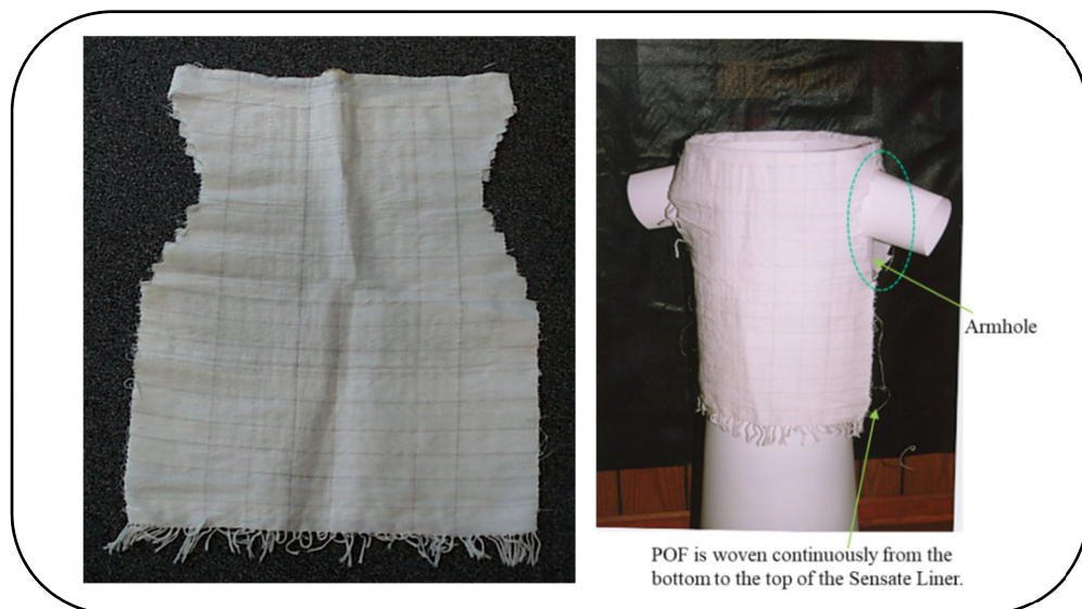
Figure 3-6 Sensate Liner \alpha -prototype
