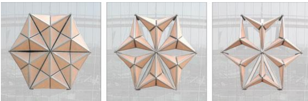
Figure 38: Mashrabiya units at unfold, midfold and maximum-fold positions
