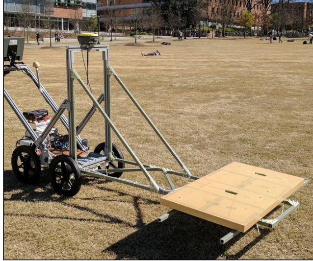
Figure 1.3: Cart-mounted wideband EMI sensor, that operates over a frequency range from 1 kHz to 90 kHz at 17 logarithmically-spaced frequencies. This sensor has one large transmit coil and four smaller receive coils.
