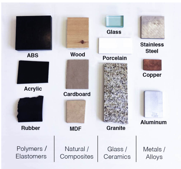
Figure 15. Twelve selected materials for real-world experiments with the 1-DoF robot
