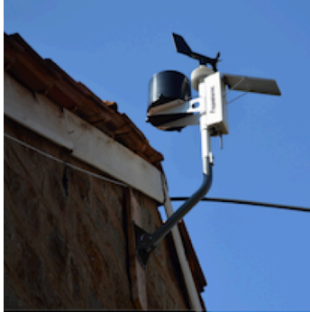
Figure 3: Image of the RainWise MK-III-LR digital weather station after it was installed on the roof of the Thika School for the Blind.
