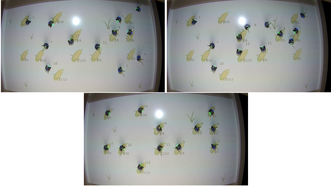
Figure 5.1: This figure shows the completion of the precision-agriculture experiment described in Section 5.5. Each pair of robots (e.g., 1 and 2) must visit a pair of crop patches, which are labeled accordingly, while avoiding collisions. This figure shows that the robots successfully visit each crop patch and avoid collisions, completing the objectives and satisfying the constraints.
