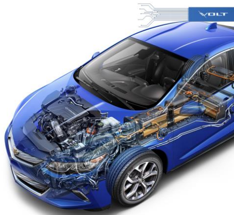
Figure 18 – Chevy Volt showing location of battery pack and motor [50]
