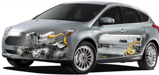
Figure 27 – Ford Focus Electric with motor and battery pack shown [57]
