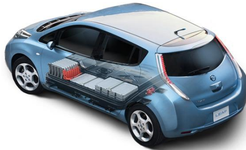
Figure 23 – Nissan Leaf with battery pack location shown [53]
