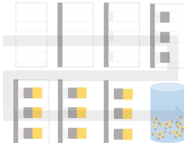
Figure 3.1 Flowchart of nanorod synthesis. A porous alumina membrane (1) is plated with metal (2), which serves as electrode. Next, silver (3), nickel (4), and gold (5) are electroplated. The membrane is dissolved (6) and the nanorods are released (7) from the sacrificial silver layer to be dispersed into a suspension (8).
