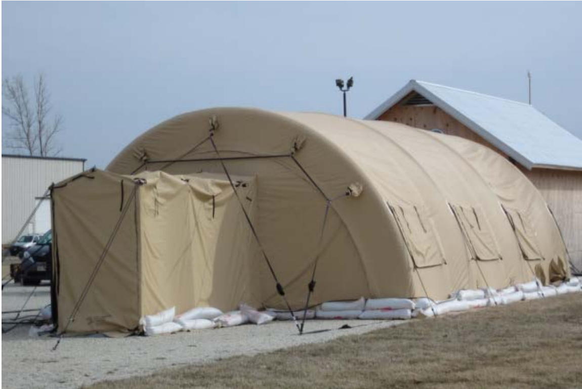
Figure 13 – Airbeam Shelter Perspective View 2: L×W×H = 20 ft × 32 ft × 11 ft [42]
