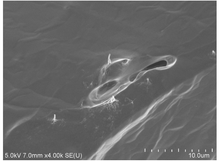
Figure 21: Void/microcrack-like structures after 691080 cycles at 10~100 N
