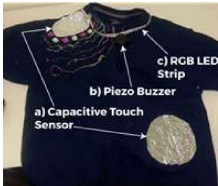
Figure 6 – One of the costume tops for the bullying-themed dance, which included: a) two capacitive touch sensors, b) a piezo buzzer, and c) an RGB LED strip
