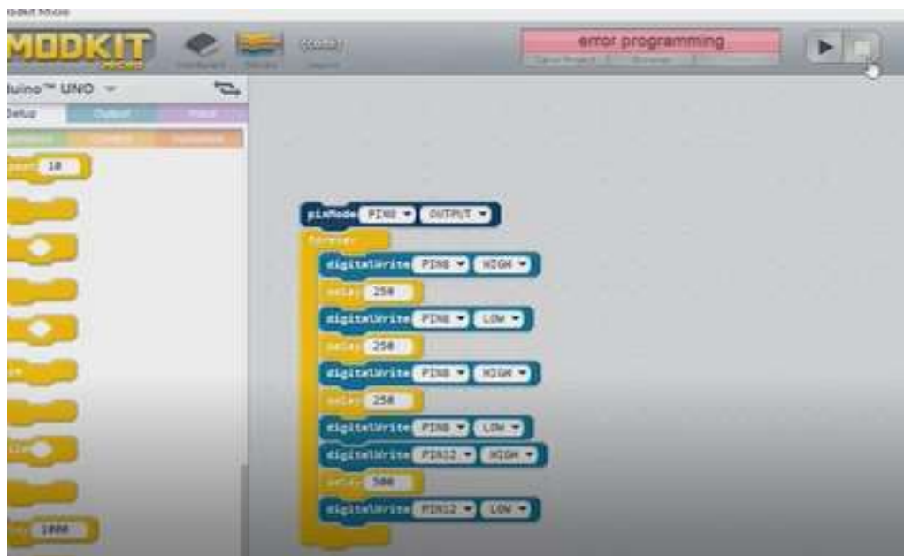
Figure 85 – Error participants would receive if they did not plug in their Arduino when programming it
