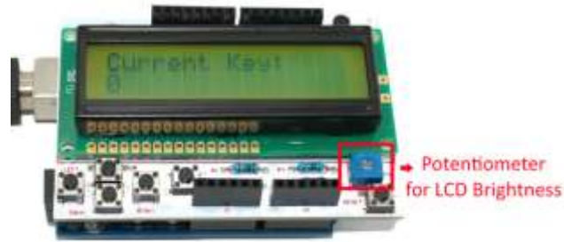
Figure 19 – LCD Breakout board that enables the user to control the brightness of the LCD using a potentiometer (“16x2 LCD Keypad Shield for Arduino Version B,” 2017).
