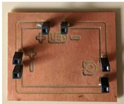
Figure 40 – Plug-and-Play Circuit Module with Variable Components used by Group 1 for Task #1. The pin headers provide positions for the LED, resistor, power and ground to be connected.
