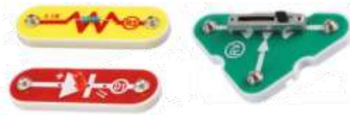
Figure 22 – Snap Circuits (“Snap Circuits,” 2017) are an example of a Level 4 Single Component Static Circuit Board
