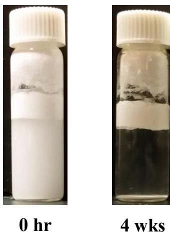
Figure 16. Foam stability test results for PS control with 5 wt% PS and no oil.
