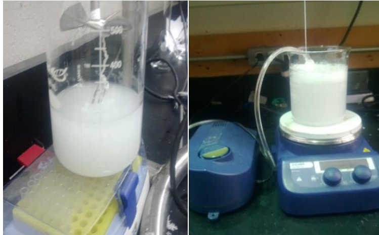
Figure 5-3 Experimental setup for (left) shear force and (right) aeration induced agglomeration and deposition.
