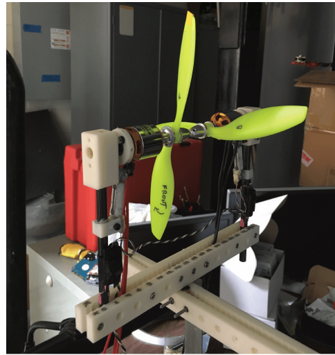
Fig. 7. Thrust stand configuration for coaxial rotors
