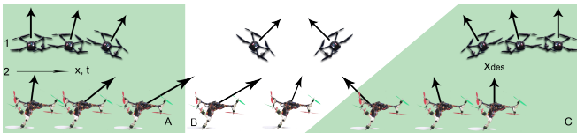
Fig. 1. Net rotor thrust for a conventional, planar multirotor (1) versus Y6sC (2) in moving to a new desired position ( x_{des} ). Regions A-C are at different times during the maneuver where the arrows indicate the force vector.
