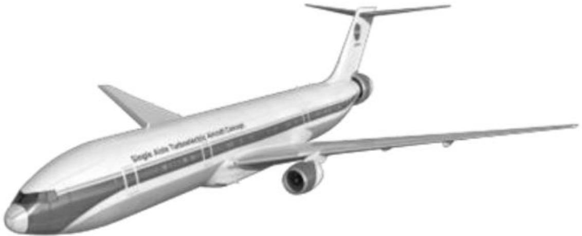
**Figure 6: STARC-ABL Concept Aircraft[29]**
