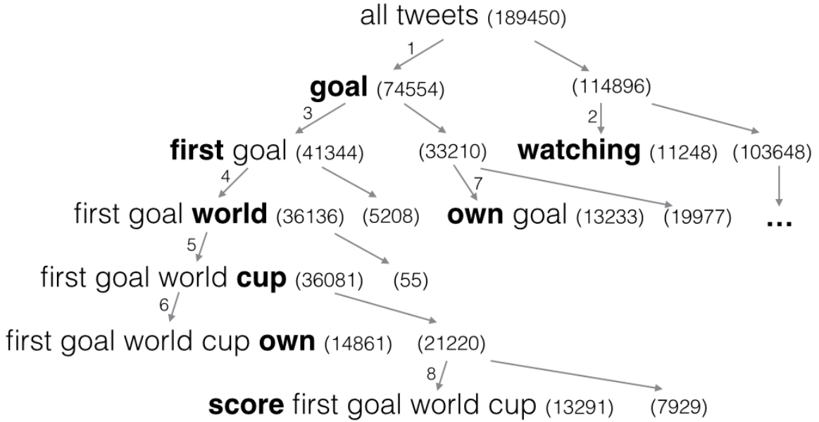
Figure 32: An example pattern generation process. The words in boldface are new words added to the parent pattern to generate the current pattern. The numbers in parenthesis are the support of each sequential pattern.
