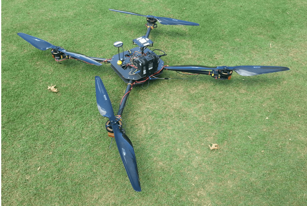
Figure 28: Eagle long endurance multirotor with 30x10.5” propellers
