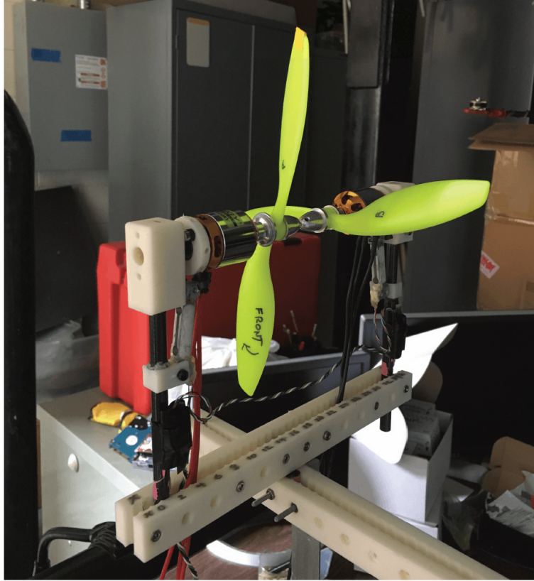
Figure 48: Thrust stand configuration for coaxial rotors
