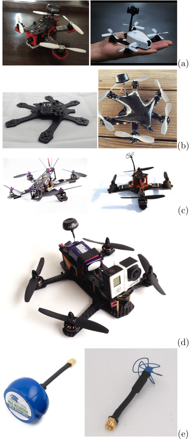
Figure 23: Configurations studied in wind tunnel, hobby multirotors made for acrobatics and racing: (a, left) 122 mm multirotor with flat vs (a, right) canopy, (b, left) 155 mm Atom chassis, (b, right) RTF 155 mm Raiju hexarotor, (c, left) 250 mm H frame ZMR vs (c, right) X frame Shrike , (d) 250 mm ZMR quadrotor with GoPro HD camera, (e, left) cased vs (e, right) uncased 5.8 GHz antenna. Thanks to Nick Willard for the photos.
