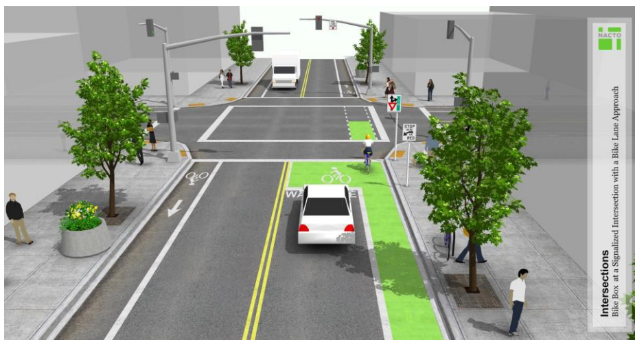
Figure 4. Example of Bike Box Installation
