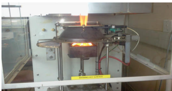
Figure 1b: Photograph of sample flaming inside the cone
