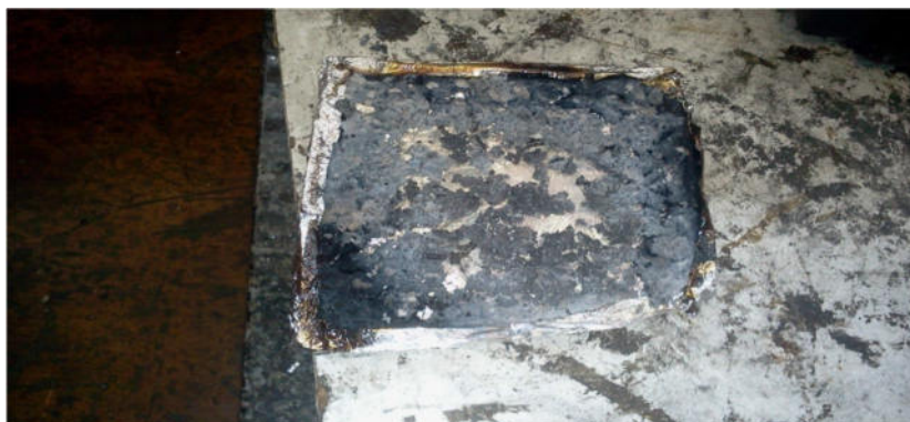
Figure 9b: Photograph of the 7.5%AH:7.5wt%BPF sample left after fire test
