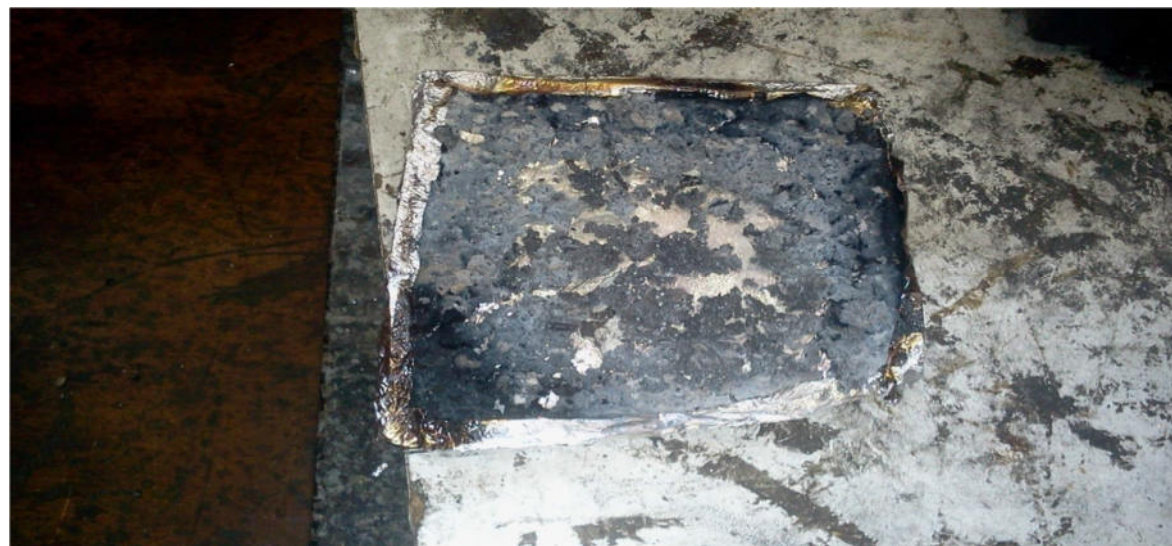
Figure 9b: Photograph of the 7.5%CHAp:7.5wt%BPF sample left after fire test
